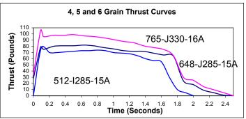
You will see that we've added a number to the front of the standard motor type code system. This number indicates the total impulse of the motor in Newtonseconds. For example, 800J360-15A is an 800Ns "J" motor, with 360N average thrust and a 15s adjustable delay
